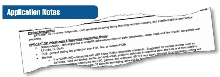
The middle portion of a datasheet contains a brief product description and type of epoxy (electrical, thermal, optical, UV, etc.) along with suggested application information.
