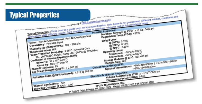
The bottom portion of the datasheet lists product properties measured by Epoxy Technology for both cured and uncured material. These properties are designed to provide an overall picture of expected performance. Application-specific testing should <u>always</u> be performed by the end user.
