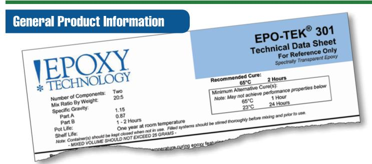
Found at the top left of a datasheet, this section specifies whether a product is **one or two components**, its' **mix ratio**, **specific gravity** as well as **pot life and shelf life**.
